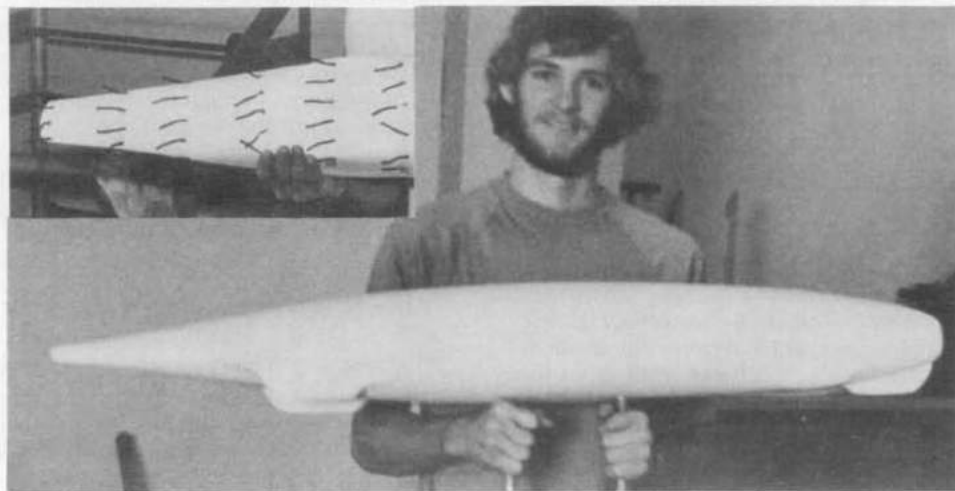
(Fig. 4) No. 1A showing how the bottom rear has been brought down to eliminate the wheel pants and large separation area. The yarn tufts are for flow visualization in the wind tunnel.
